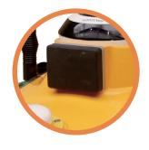
Millimeter wave radar
